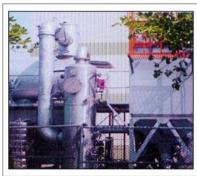
Packaged Small-scale Incineration System Capacity : 500 kg / hr
